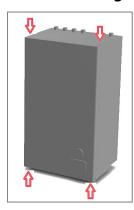
To access the wiring board, the front panel must be removed.
