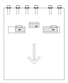
3. Slide the pre-installation rig to the right by 30 mm
